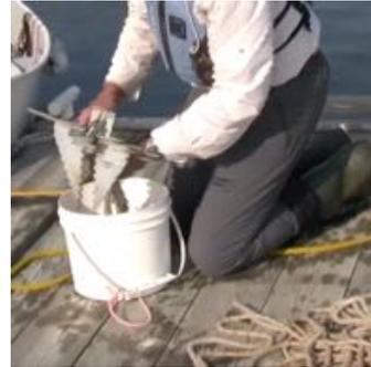
Place the remainder of the line loosely in a second container- first in, last out.
