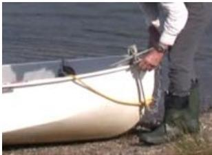
On landing, place your anchor on the boat's bow. If needed use a blanket, or padding to protect the surface. Make sure the padding is secure, or it will get dragged into the water
