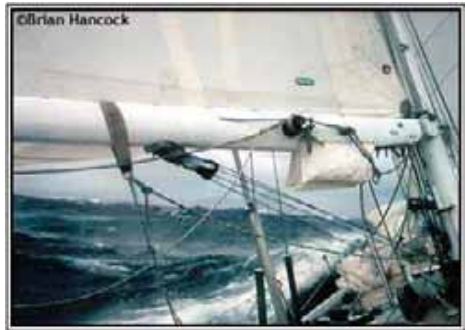
The preventer, seen on this former Whitbread Race boat just aft of the vang on the boom, keeps the boom from becoming lethal should the boat unexpectedly jibe.
