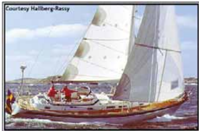
The reef points and reinforcement patches on this mainsail are clearly visible. This sail would be described as having two full sets of reef points.
