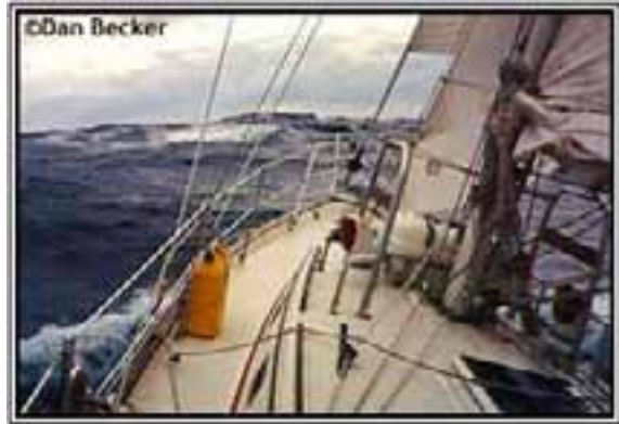
Feathering up into the wind in heavy air and big seas can take some of the strain off the rig and the hull as you work through a difficult seaway.
